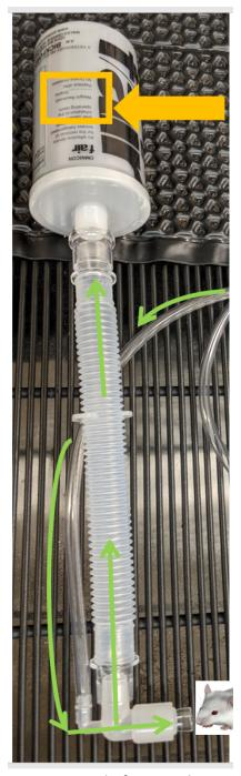
Charcoal canisters are used to absorb waste isoflurane gas. Weigh the canister before the first use to give starting weight and record on the side of the canister.
